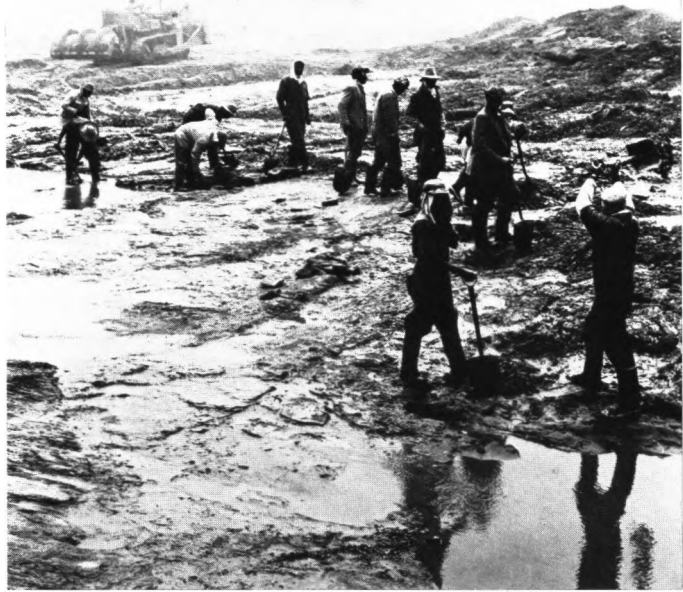
58 A more detailed view of beach mining, showing a machine scooping up gravel in the background while miners clear the remainder by hand to expose bed rock
